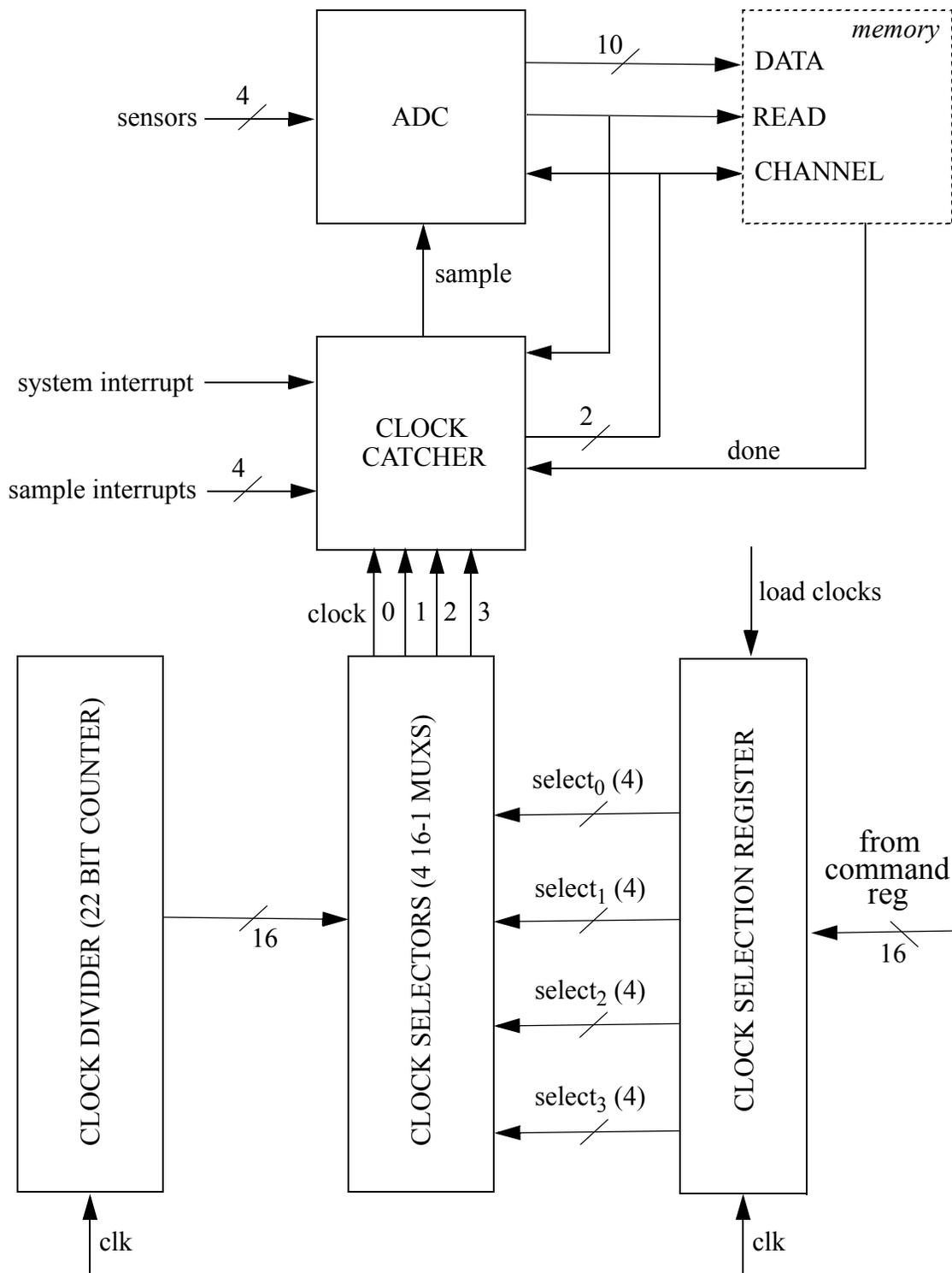
FIGURE 8. Sample and Delay Controller
