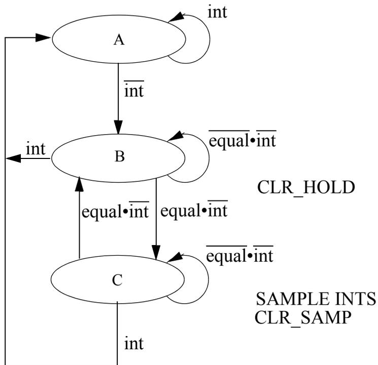
FIGURE 7. ADC Controller
