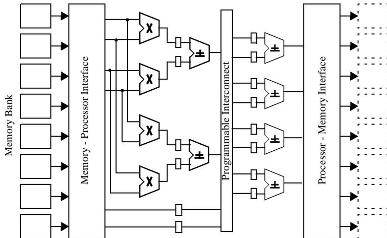
Figure 2: Prototype chip architecture
